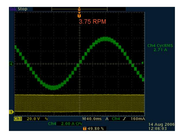
**3.75 RPM** picture: Note the sine current quatified every 9 electrical degrees. The 20kHz PWM duty cycle stays between 45 to 55 percent (yellow trace). Motor motion is very smooth, the microstep rate is 125 Hz, a frequency which is above the motor's mechanical cutoff frequency of 80Hz.
